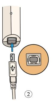
When positioned correctly, the cord will slide in gently. Do not force.
