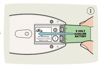
c. Slide the 9-Volt Alkaline battery into the case and push down. Slide the cover back onto the unit.
