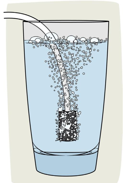
6. At the end of a timed session, the unit will beep, all the LED lights will flash, and the air pump will continue to operate for an additional 10 seconds to purge the ozone from the tube. The unit will then turn itself OFF.
