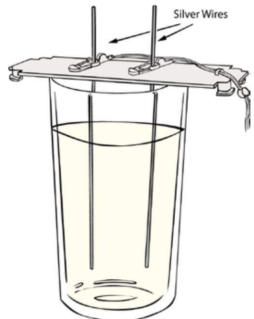
The next step of course is to simply turn the unit on. You turn the unit on and the green light comes on and right away you should see the orange light for silver. That tells us that there must be a current flow through the silver wires, through the water and into the unit and turning the light on. We are actually making Colloidal Silver right now.
