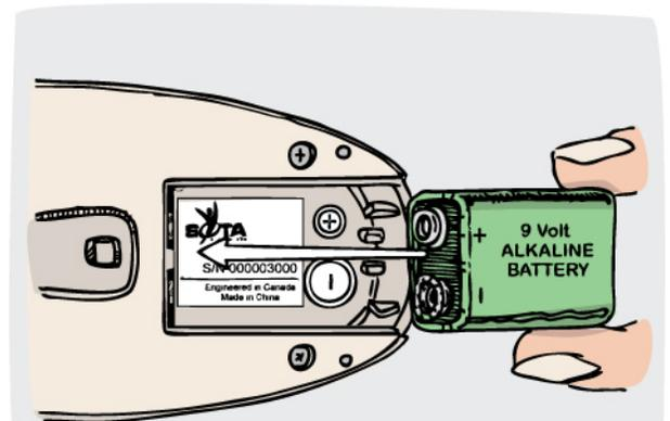
On the battery, of course, there are two terminals—the bottom one is the lower negative terminal, the larger one, and at the top is a smaller positive terminal. You simply line them up in this fashion. Slide it in, click it into place, put your battery lid back on, turn the unit over, and I'll turn the unit on. And you should see a green ON light. That tells me the unit is ready to go and the battery is working just fine.
